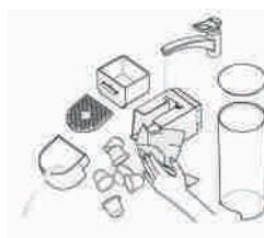
**① Empty the drip tray,** the drip base and the capsule container every day. Also remove the water tank with its lid and clean them all with odorless detergent and rinse with warm / hot water.
